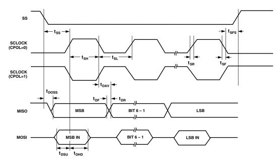
Figure 59. SPI Slave Mode Timing (CPHA = 0)
